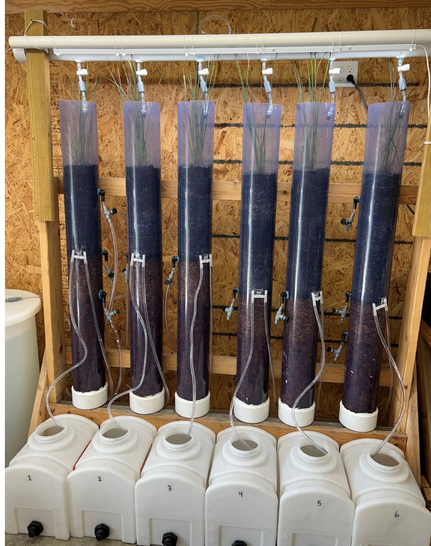
Experimental Setup with Supply Tank, Columns and Collection tanks
