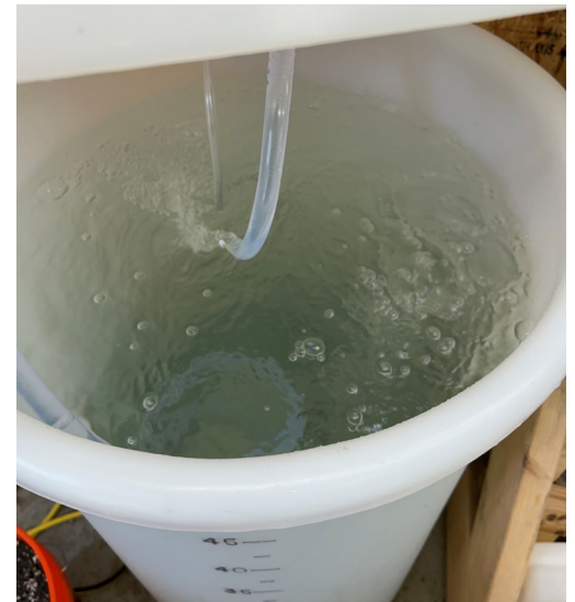
Supply Tank with Feed Pump and Bubbler to keep inflows agitated
